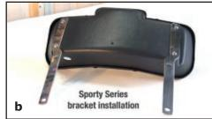
Attach the two provided brackets to the radio. Use the screws removed from the radio earlier to install the brackets. Insert and tighten the shorter top screws (c). The longer screws will be used in the bottom holes. Loosely put them in the holes now to keep them handy (d).
