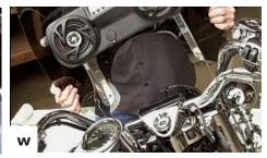
(x) Take the two-pin power plug on the audio wiring harness and connect to the socket on the bottom of the audio system.
