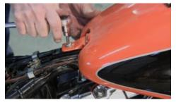
Connect the wiring harness to the battery under the seat. The orange cable, goes to the positive terminal (u), then the
