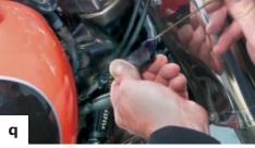
Feed the harness up the handlebar(r) to the audio system and zip-tie the harness to the existing bike wiring using
