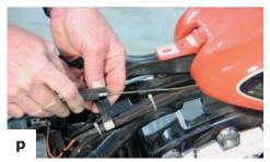
Use the hanger to pull the harness from the front end of the gas tank, until the taped plug is through the tank
