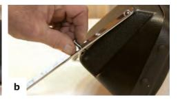
Remove the five OEM windshield screws and acorn nuts from the windshield frame. The three indicated
