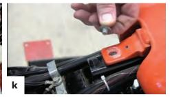
Once released you can lift the tank(1) and block it up an inch or two using anything handy, such as a screwdriver (m).
