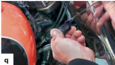
Feed the harness up the handlebar (r) to the audio system 2 or 3 ties in front (s) of the tank and behind the tank (t). and zip-tie the harness to the existing bike wiring using
