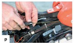
Use the hanger to pull the harness from the front end of the gas tank, until the taped plug is through the
